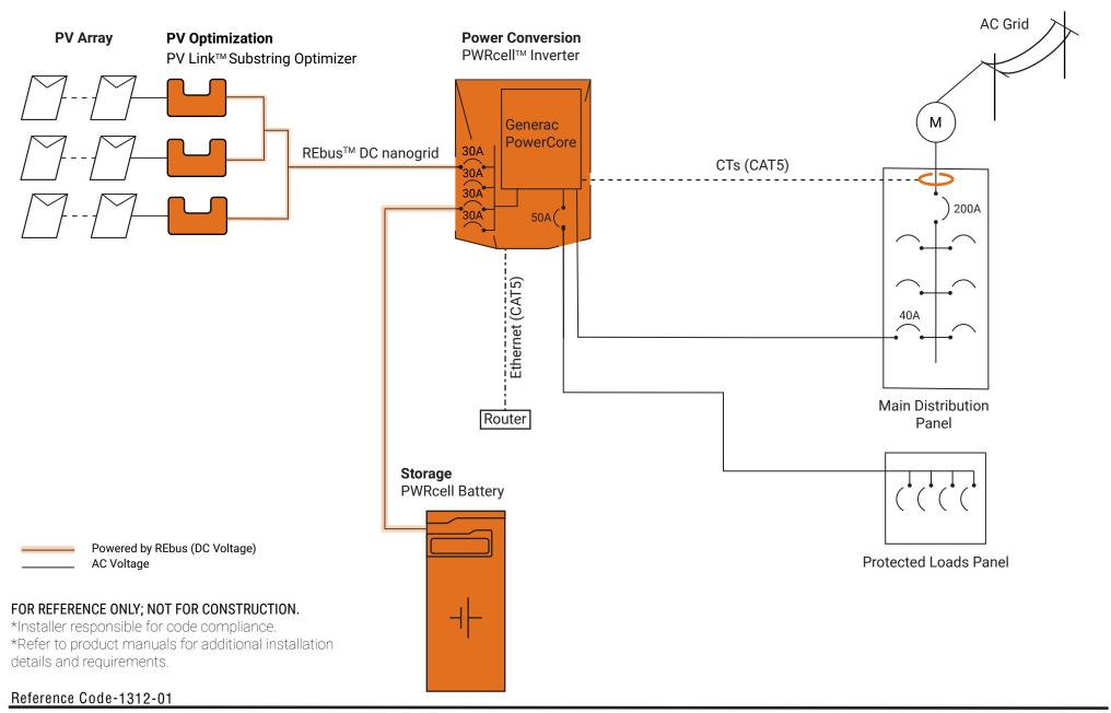
This design shows a PWRcell system with a Protected Loads panel to provide backup power to loads.
