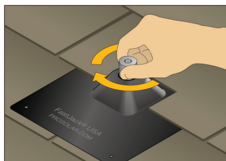
Step 6: Tighten FastJack® post into base
