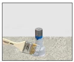
STEP 6: Apply M-1 Sealant to post. (Optional: Place painter's tape around post approximately 3" above roof.)
