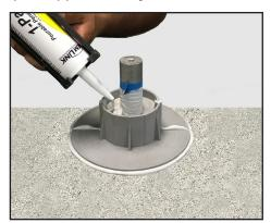
STEP 9: Fill E-Curb with 1-Part filler and remove tape.
