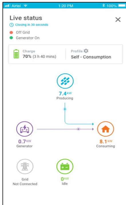
Figure 24: Live status screen with generator
