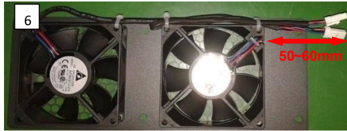
Figure 8-1 Replacing Cooling Fans
