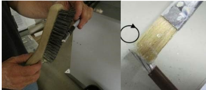
Figure 3-38 Preparing Aluminum Wires Prior to Connecting
