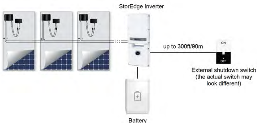
Figure 49: System connected to an external shutdown switch
