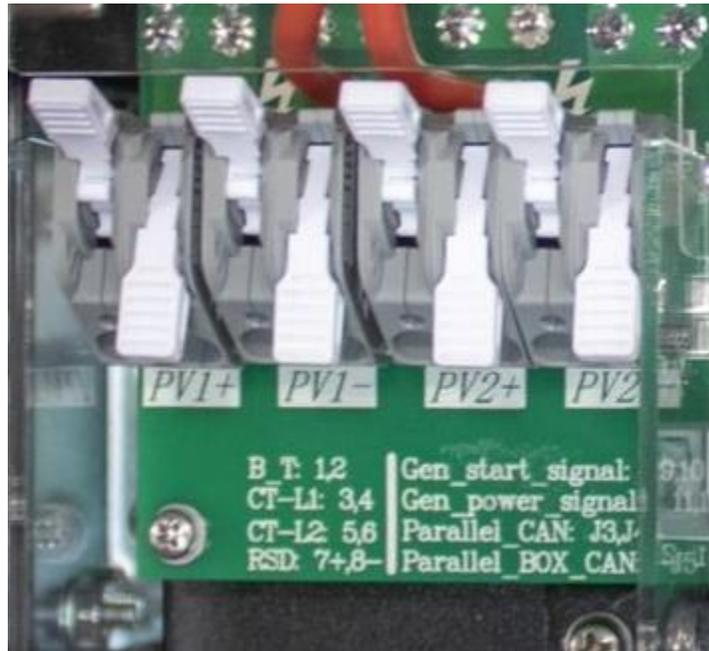
Figure 17.0 - PV Array Connection Points (DC Coupled Systems)
