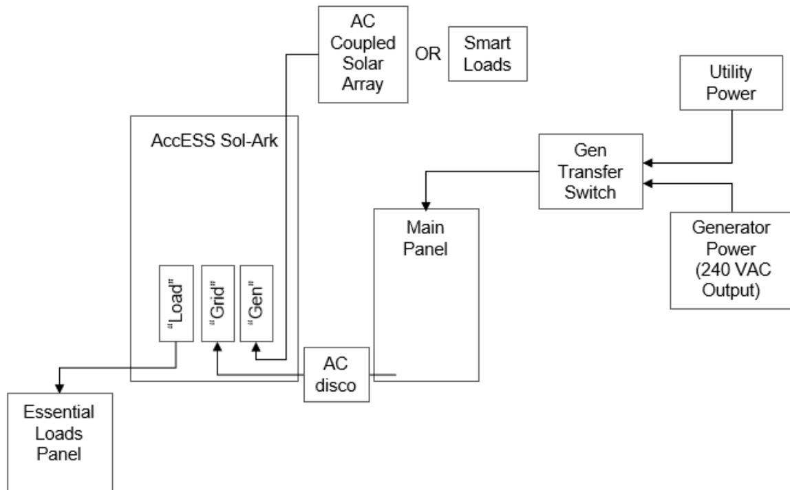
Figure 15.0 - Generator Wiring in Grid-Connected AC Coupled Systems
