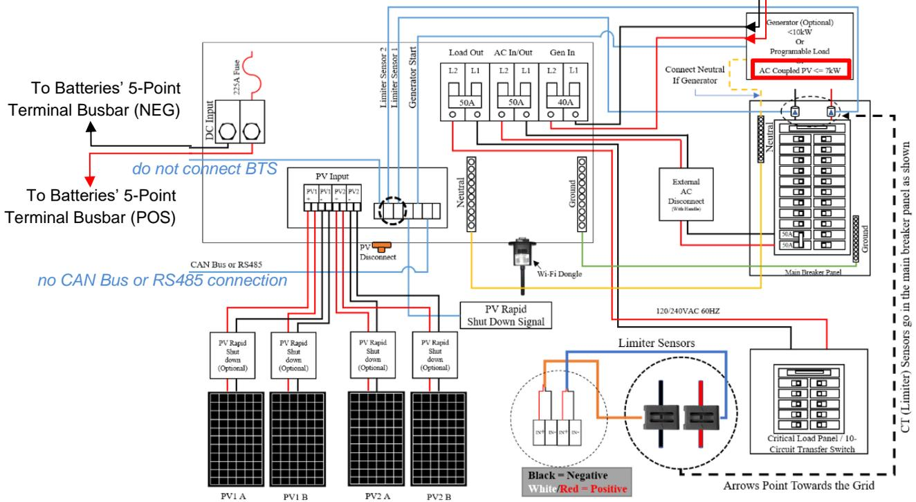
Figure 13.0 – AC Coupled ACCESS Sol-Ark Wiring Diagram
