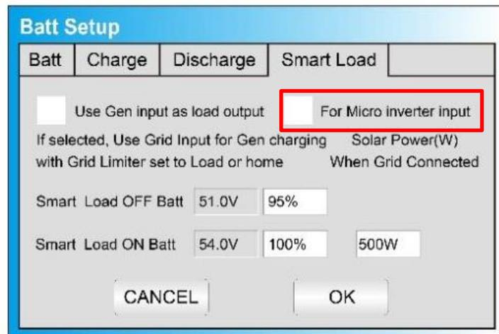
The Sol-Ark-8K is limited to a maximum of 7 kW of AC Coupled solar PV, and the Sol-Ark-12K is limited to 7.6 kW of AC Coupled solar.
