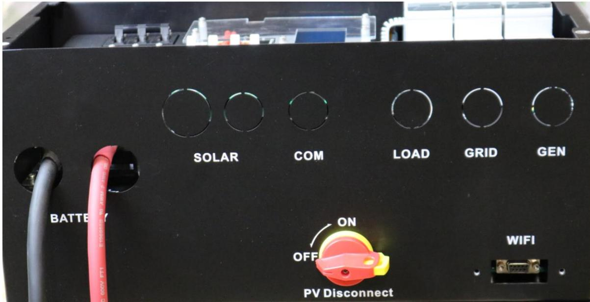
Figure 19.0 – Sol-Ark PV Disconnect in DC Coupled Systems
