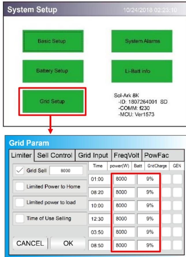
Figure 21.0 – Limiter Tab in Grid Setup Menu
