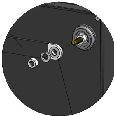
**Figure 10.0 – Interconnecting Busbars Secure to the Batteries' Terminals**
