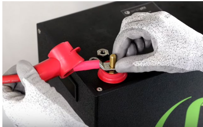
Figure 11.0 – Lugs Wired in Direct Contact with Current Carrying Battery Terminal
