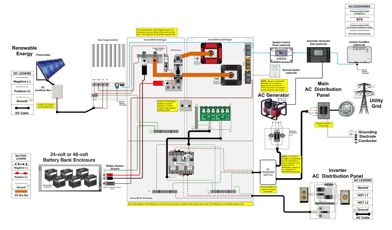
Figure 3-4 Single-Inverter System Renewable Energy (Solar) Wiring
