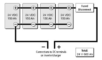
Figure 1-19 Batteries Connected in Parallel
