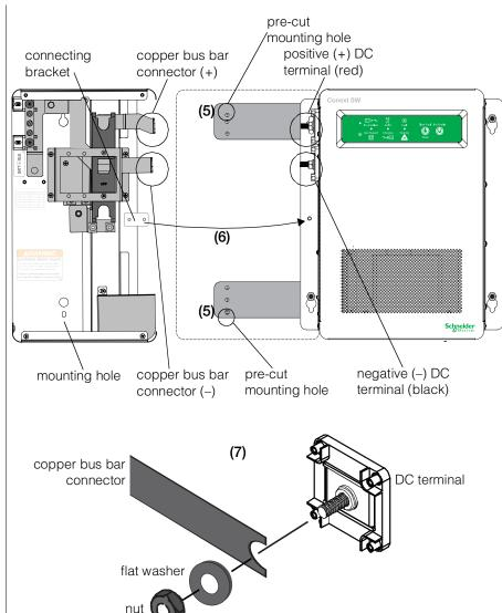
Figure 1-12 Installing the DC Switchgear
