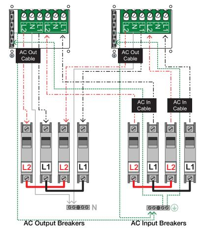
The Input and Output Neutrals are electrically tied at the inverter terminals. Only a Neutral wire (from the AC Out cable) is necessary from each inverter.
