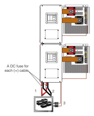
Figure 1-17 Connecting Battery Cables
