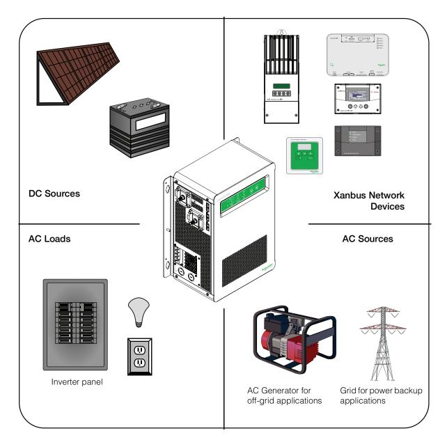
Figure 1-8 AC, DC, and Network Components
