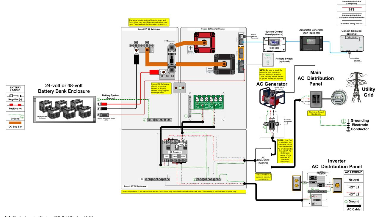
Figure 3-2 Single-Inverter System (Off-Grid/Backup) Wiring
