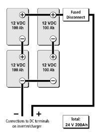
Figure 1-21 Batteries in Series-Parallel Connections
