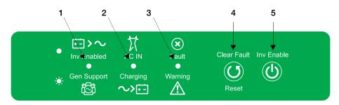
Figure 1-3 Front Panel Buttons and Status LEDs
