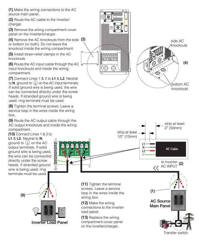
Figure 1-11 Conext SW AC INPUT and OUTPUT Connections
