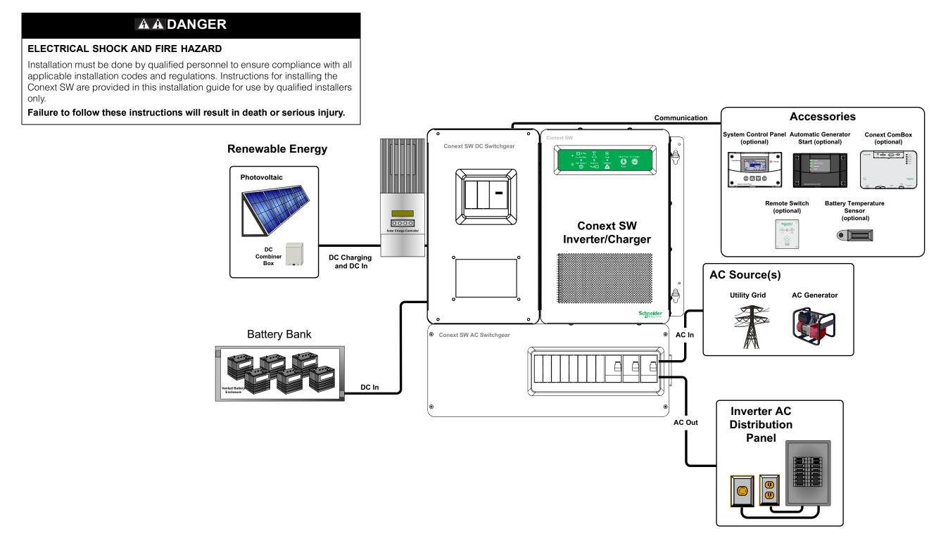
Figure 3-3 Single-Inverter System Renewable Energy (Solar) Overview
