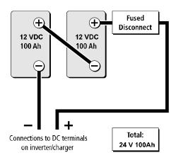
Figure 1-20 Batteries Connected in Series
