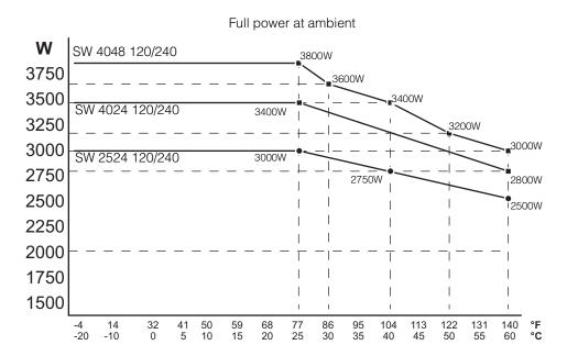
Figure 2-1 Output Power versus Temperature Derating Graph
