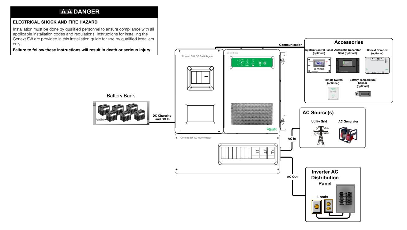
Figure 3-1 Single-Inverter System (Off-Grid/Backup) Overview
