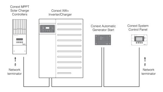
Figure 4-1 Xanbus Network System (Example)
