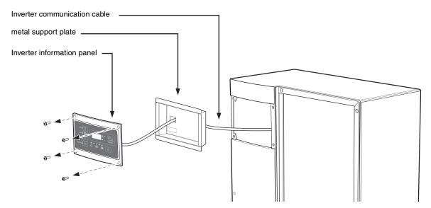
Figure 5-2 Inverter information panel removal
