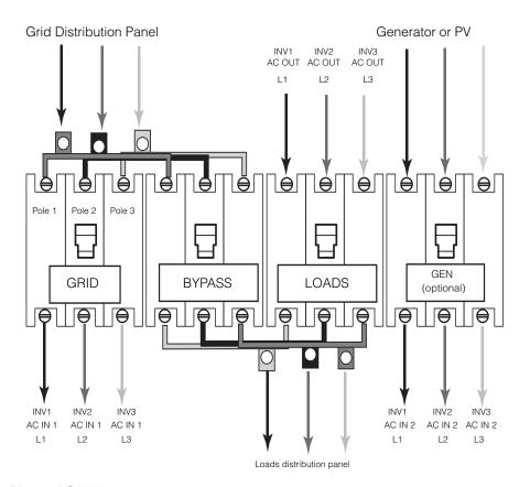
Figure 3-33 PDP Three-Phase AC Wiring
