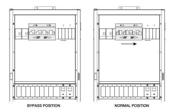
Figure 3-26 Installing the custom designed bypass interlock plate
