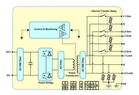
Figure A-6 Conext XW+ Block Diagram
