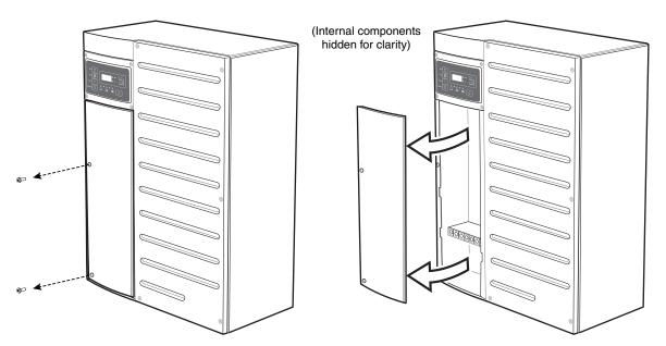
Figure C-2 AC access panel removal
