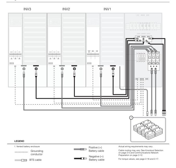
Figure 3-27 DC Connections for a Triple-Inverter System
