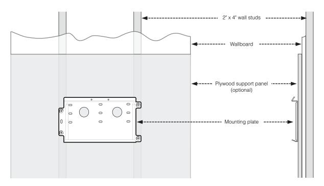
Figure 2-5 Mounting plate centered on wall studs
