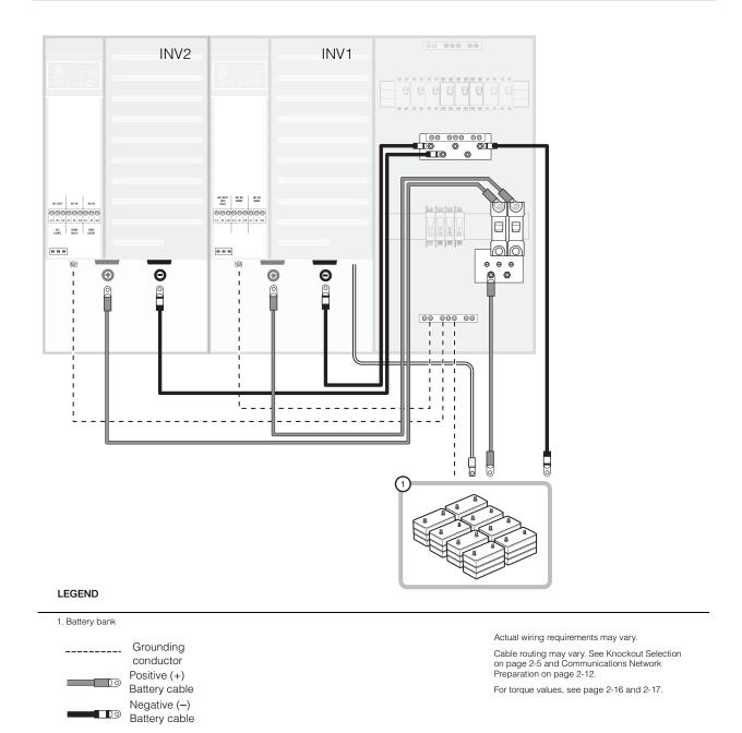
Figure 3-23 DC Connections to Dual Inverter
