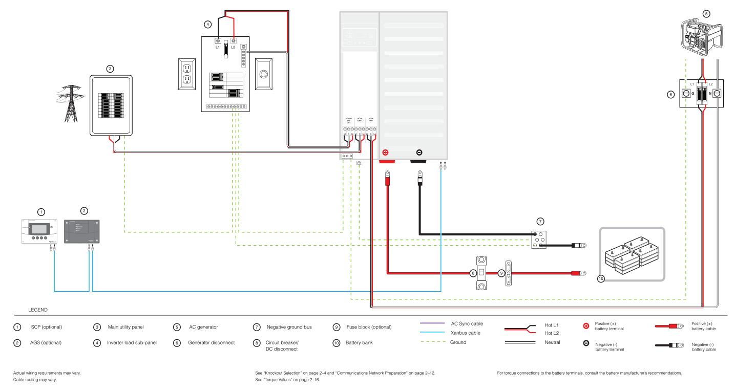
Figure B-1 Single-Inverter System (Backup Only) Without a Conext XW+ Power Distribution Panel
