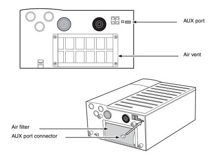
Figure 2-3 Air Filter and AUX Port Connector Installation
