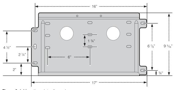
Figure 2-4 Mounting plate dimensions
