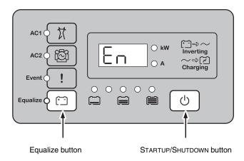
Figure 3-18 Enabled mode
