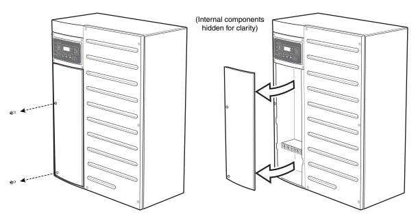
Figure 3-1 AC access panel removal
