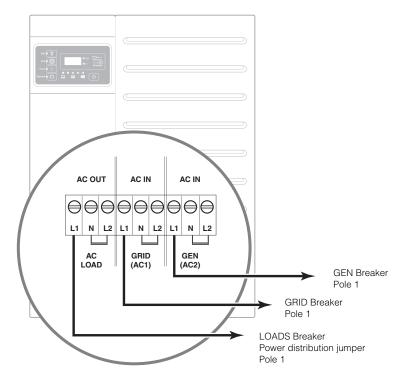
Figure 3-34 Inverter/Charger Three-Phase AC Wiring
