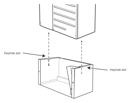
Figure 2-8 Conduit Box keyhole alignment
