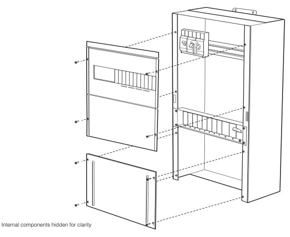
Figure 3-2 Conext XW+ Power Distribution Panel faceplate removal
