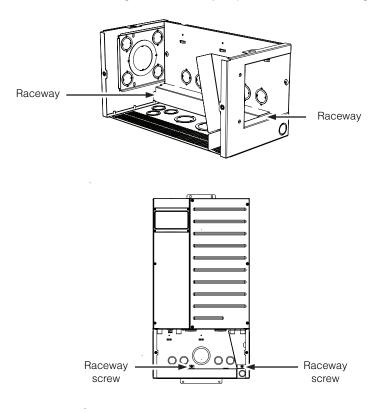
Figure 4-5 XW+ Conduit Box raceways
