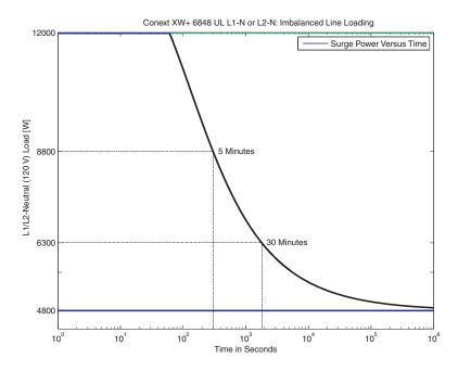
Figure A-1 Conext XW+ AC Overload Capability
