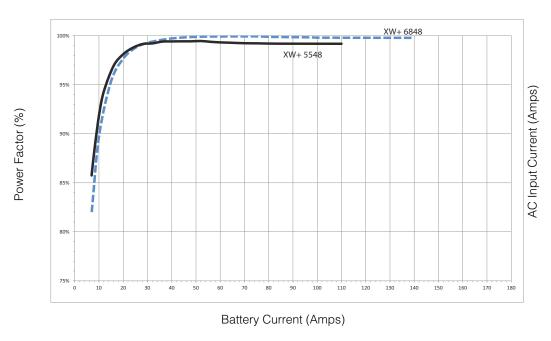
Figure A-5 Charging Efficiency (Power Factor)
