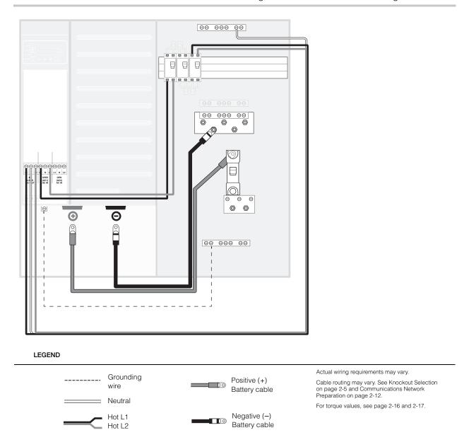
Figure 3-12 Wiring the Conext XW+ Power Distribution Panel to the Conext XW+ Inverter/Charger
