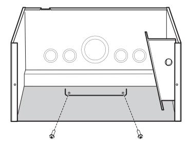
Figure 2-9 Wall-mounting the Conduit Box
