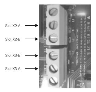
Figure C-4 Slot Locations on X1 and X2 Connectors
