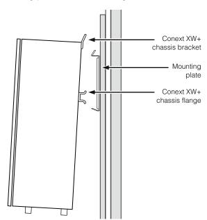
Figure 2-7 Wall-mounting the Conext XW+
