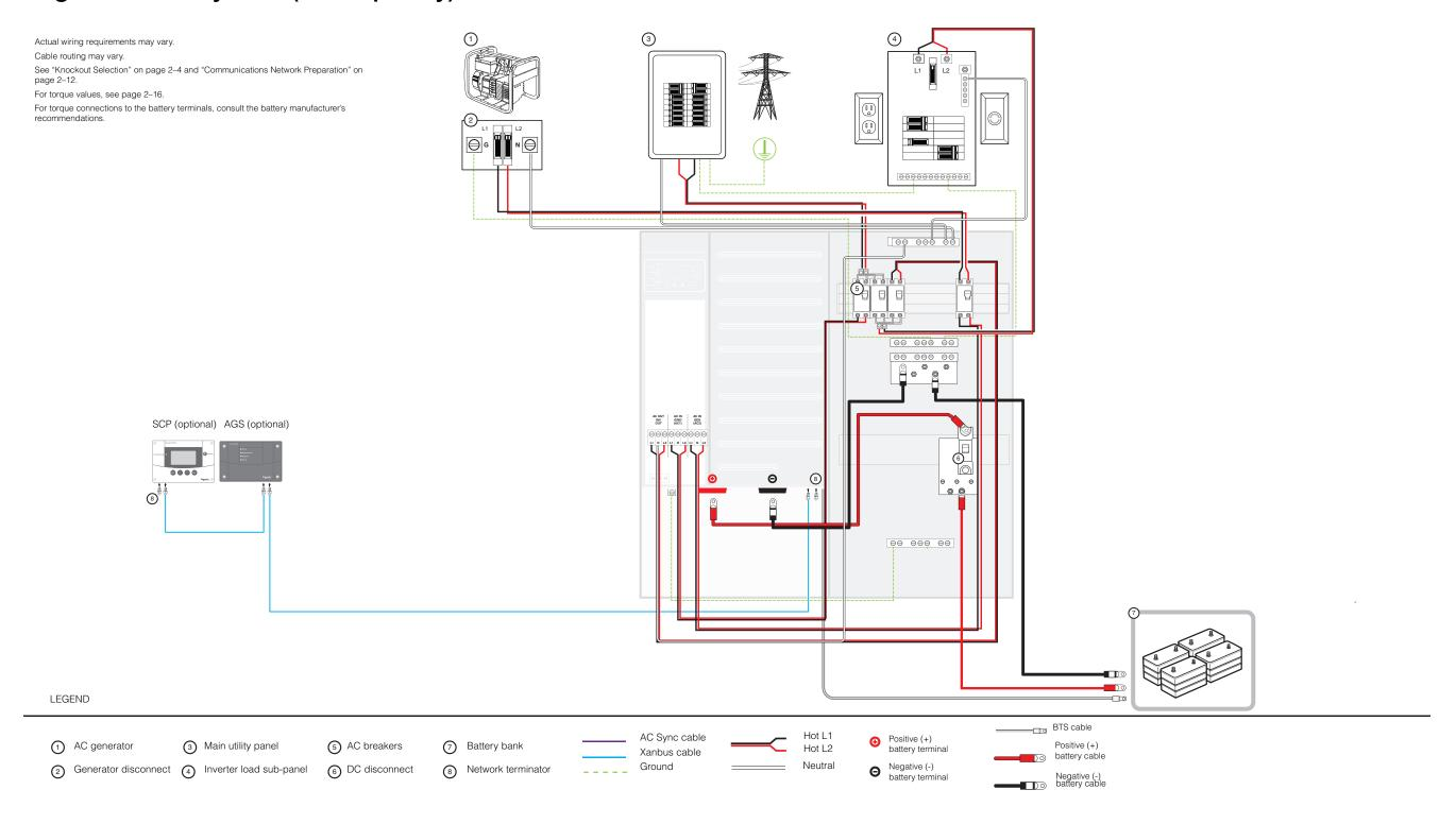
Figure B-2 Single-Inverter System (Backup Only) With a Conext XW+ Power Distribution Panel
