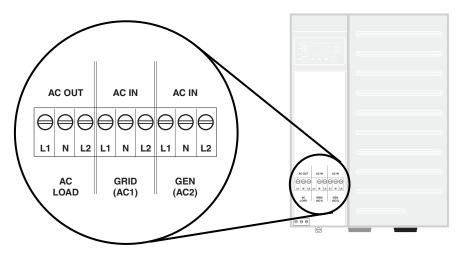
Figure 3-10 AC terminal block
