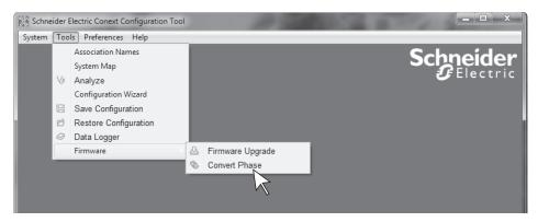
Figure C-7 Upgrading the firmware
