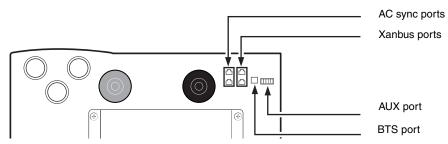
Figure 4-4 Conext XW+ Inverter/Charger communication ports
