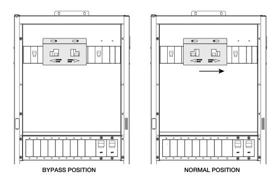
Figure 3-35 Installing the custom designed three-phase bypass interlock plate
