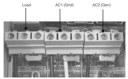
Figure C-6 Jumper Locations and AC Cable Configuration on AC Ports
