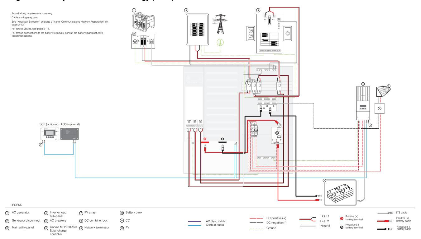
Figure B-3 Single-Inverter System Renewable Energy (Solar)
