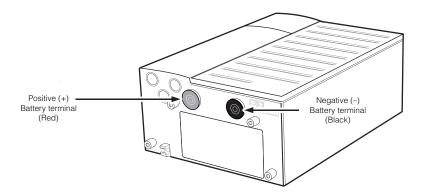
Figure 3-7 Battery terminals (bottom of Conext XW+)
