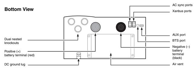
Figure 1-2 Conext XW+ Inverter/Charger Features
