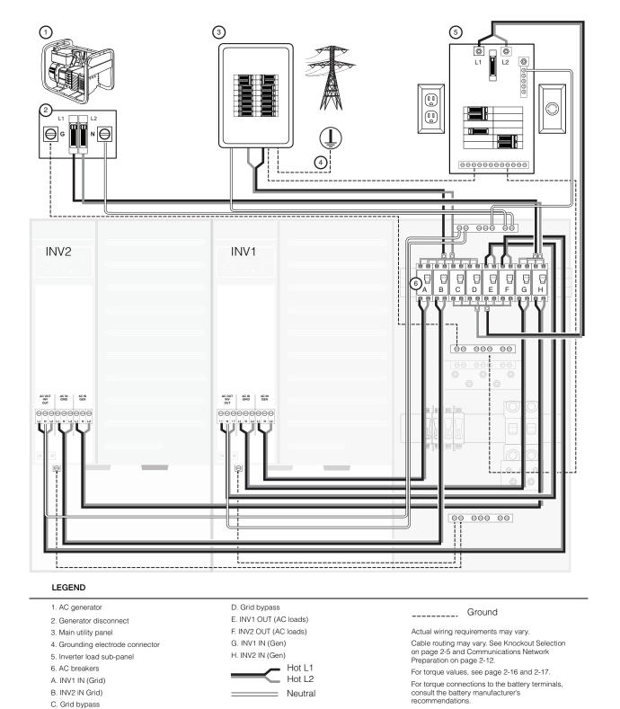
Figure 3-25 AC Wiring for Dual-Inverter Systems
