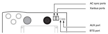
Figure 3-3 Conext XW+ Inverter/Charger communication ports
