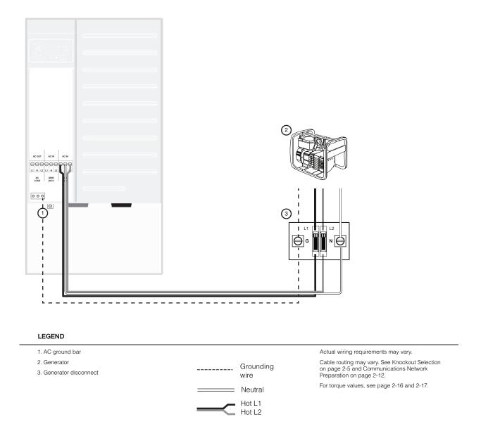
Figure 3-40 Generator Wiring directly to the Inverter (No PDP)
