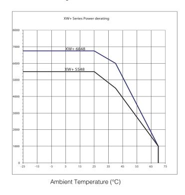
Figure A-2 Output Power Versus Ambient Temperature
