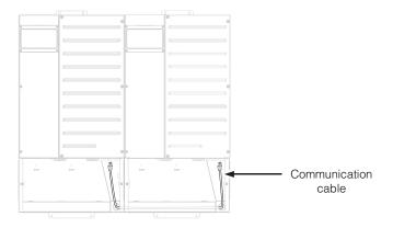
Figure 4-6 Installing the AC sync and Xanbus cables
