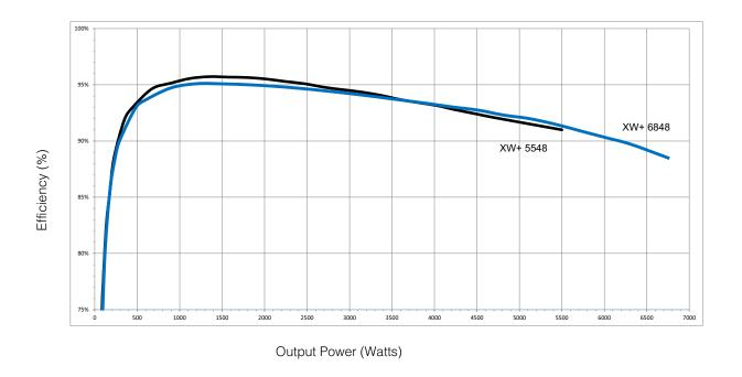
Figure A-3 Inverting Efficiency (Typical)
