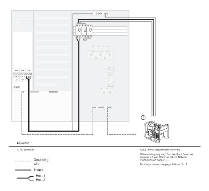
Figure 3-14 Wiring the PDP to a Generator (Off Grid)
