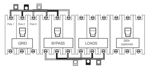
Figure 3-32 Power Distribution Jumper Installation (Three-Phase)
