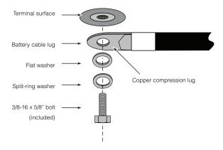
Figure 3-8 Battery cable connection
