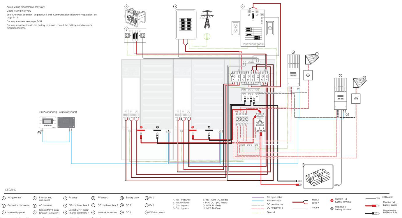
Figure B-4 Dual-Inverter System Renewable Energy (Solar)
