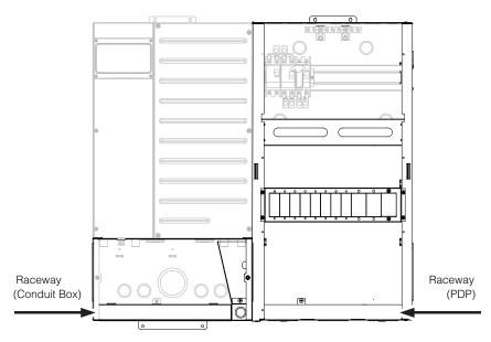
Figure 2-11 Example of raceways in a single-inverter system
