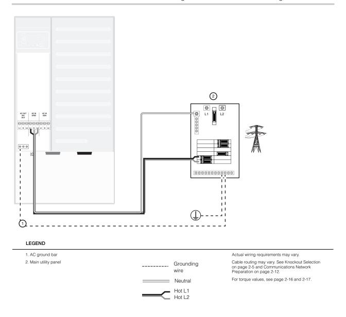
Figure 3-41 Utility Wiring to the Inverter Input (No PDP)
