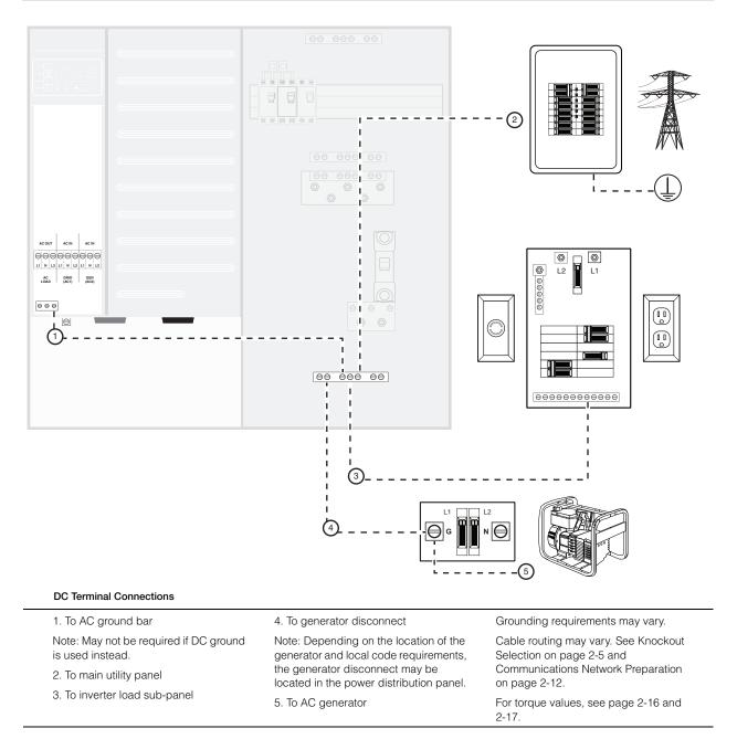
Figure 3-5 DC Grounding Using a Conext XW+ Power Distribution Panel
