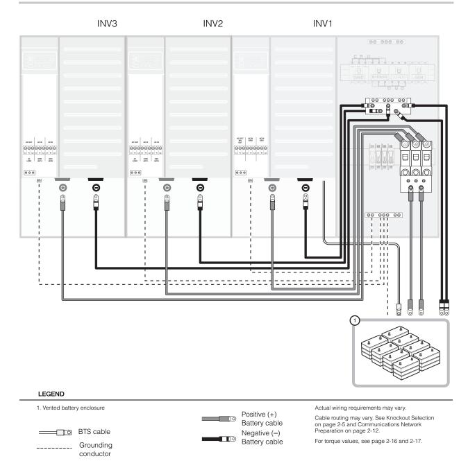
Figure 3-31 Three-Phase DC Wiring
