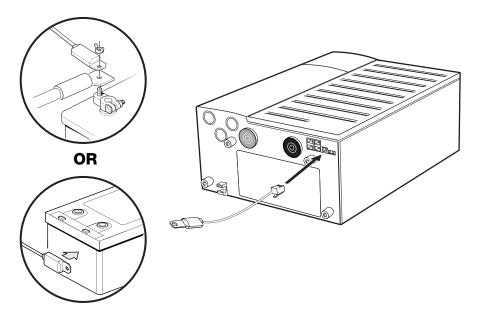
Figure 3-6 Battery Temperature Sensor Installation
