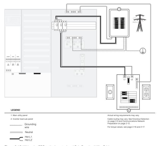
Figure 3-15 Wiring the PDP to the Inverter Load Sub-Panel or Utility Grid
