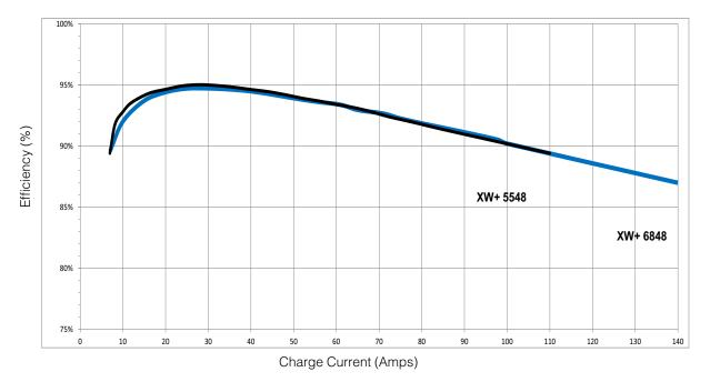
Figure A-4 Charging Efficiency (Typical)
