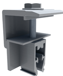
Image 2.4.9 Universal end clamp [8 ft-lbf (11 N-m)]
