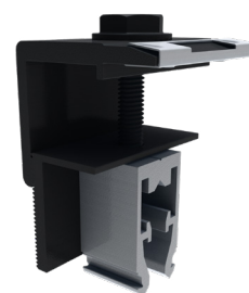
Image 2.4.10-1 Universal end clamp w/WEEB-BMC [8 ft-lbf (11 N-m)]
