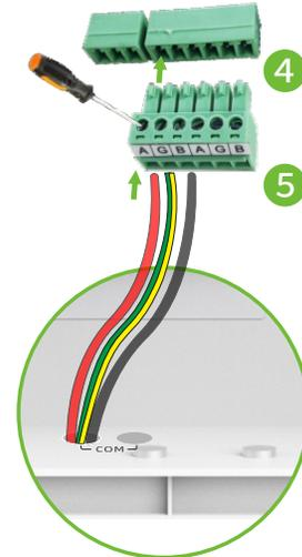
1. Use the four-core or six-core twisted pair cable and strip 0.31 inches (8 mm) of the cable insulation.
