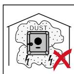
The inverter is essentially designed to be dustproof (Type 4X). In areas of high dust accumulation, dust deposits may collect on the cooling surfaces, and thus impair the thermal performance. Regular cleaning is required in this case; see the chapter headed [Operation in dusty environments](#) on page 125. We therefore recommend not installing the inverter in areas and environments with high dust accumulation.
