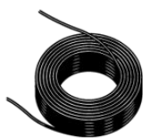
Copper conductors- No. 8-3 AWG (11 mm or 7/16" strip length) (rated at 90°C) for terminals
