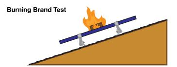
A burning wooden block is placed on module as a fan blows at 12 mph. Flame cannot be seen on underside of roof within 90 minutes.
