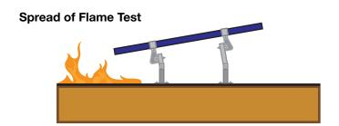
Flame at southern edge of roof is aimed up the roof as a fan blows at 12 mph. The flame cannot spread 6 feet or more in 10 minutes.
